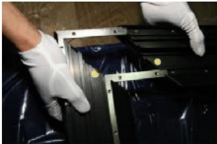
Connect the frames (A2, A3) together. Repeat this process for the rest of the corners.
