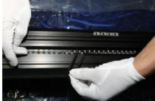
Remove the rubber band used for fixing the hooks.
