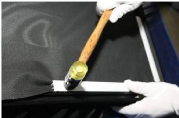
If the depression bars cannot be pushed in place with fingers, use the included soft hammer (P3).
