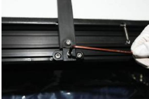
First take out the shaft pillars (P8) and install them at the 1/4 positions (see diagram) of the screen. Place M6 screws (P7) through the connectors' holes and connect with the square nuts already in place inside the frame's grooves. Take out the support shafts (A8) and fasten them with M6 screws (P7).
