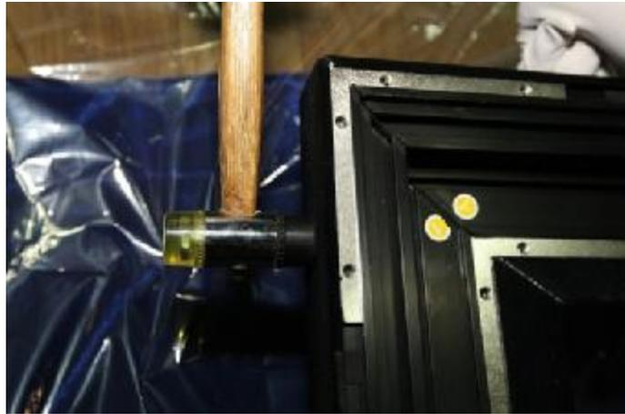
If there is a gap in the frame junctions, use the soft hammer (P3, included) to correct it.
