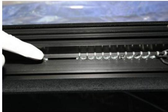
Attach the screen hooks carefully onto the perforated locations of the screen (A4) one by one.
