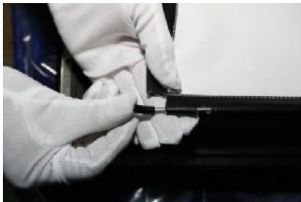
When the steel wire has been inserted properly, refit the end of the steel wire with the plastic sleeve.
