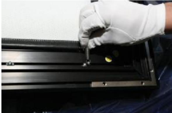
Take out the draw springs (P6) and use a pair of needle-nose pliers (P2) to pull them toward the screen and hook them into position.
