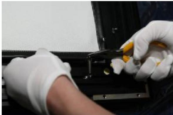
First, fix the four corners of the screen, with preferably two draw springs on each side. Then adjust the screen's position accordingly.
