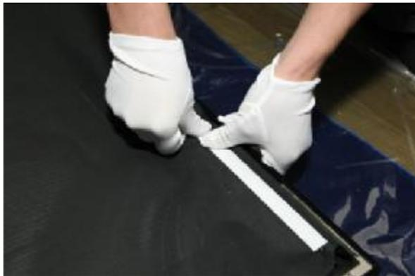
Use depression bars (P9) to fix the black backing fabric (A4) tightly in place, and make sure the installation is symmetrical. Then stretch the black screen and push down the depression bars.
